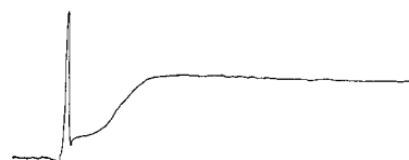
FIGURE 13: Sedimentation velocity experiment on polylysine-DNA complex. This scanner tracing was taken about 12 min after reaching a rotor speed of 2600 rpm. Temperature was about 22^\circ .
